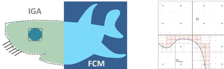
**Fig. 1** Geometry principles of isogeometric analysis and the finite cell approach (left), composed adaptive numerical integration scheme for immersed boundaries (right).
