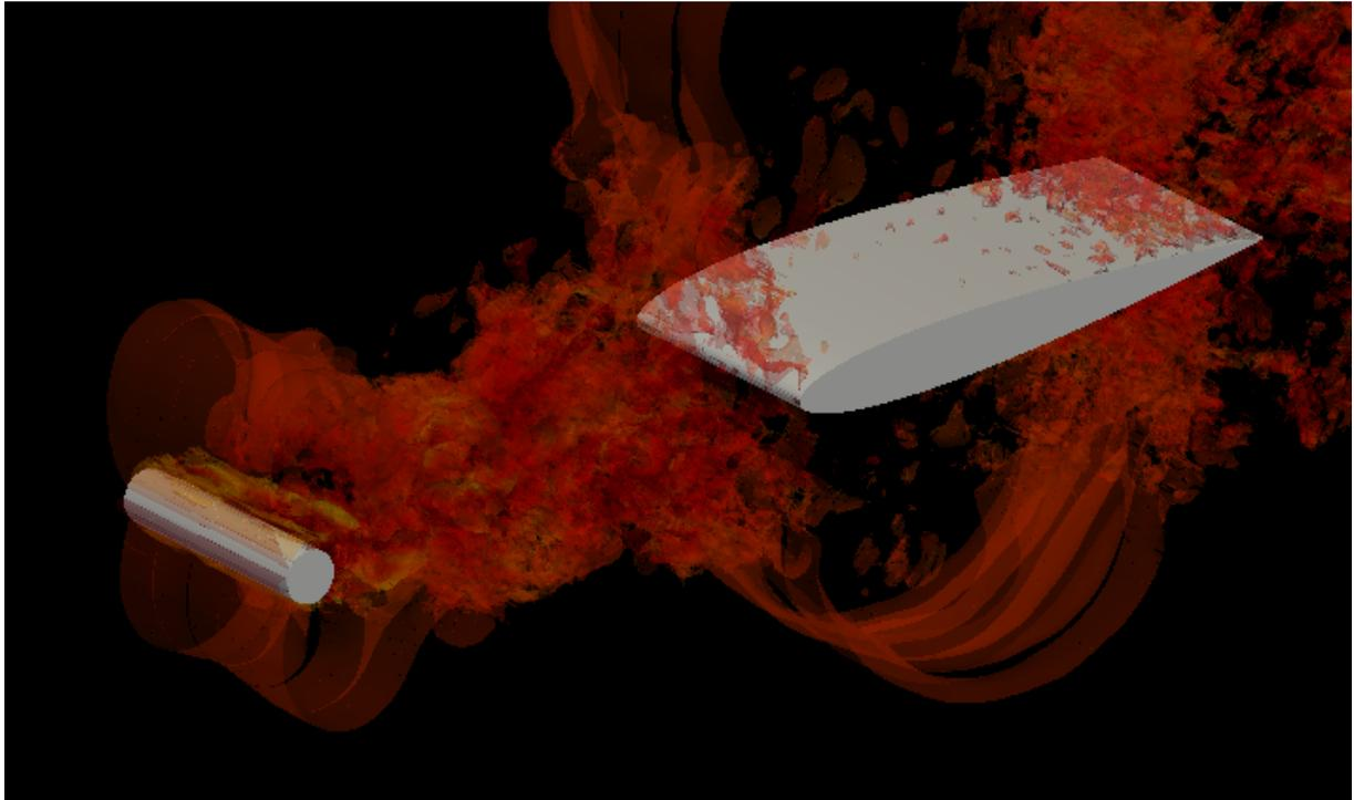
**Fig. 2** Instantaneous pressure isosurfaces,  $Re=480,000$ ,  $Ma=0.21$ . Coloured by velocity magnitude.
