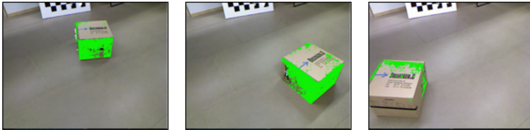
Fig. 6: Kinematic morphing network predictions (green box) overlaid with point clouds from a Kinect camera.
