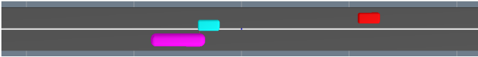
Fig. 1: The ego vehicle (cyan) wants to overtake but cannot observe if a vehicle arrives in the opposite direction because of the truck.
