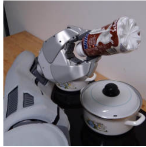
Fig. 9. Failed grasp using the AG interface. The grasp failed because the object was grasped from above for Task 3 - pour from a bottle into bowl.
